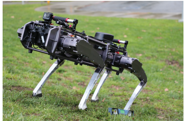
Fig. 1: The Vision 60 quadrupedal robot (V3.9) standing on a 20^\circ \sim 25^\circ sloped lawn.
