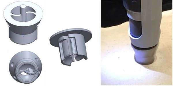
Figure 7. Curved teeth array bit and lid design (left) and fabricated integrated into a testbed (right)
