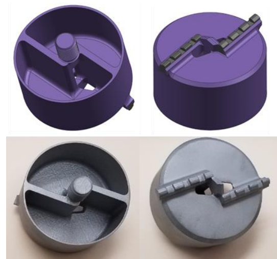
Figure 5. Cylindrical bit with linear teeth array design (top two pictures) and 3D printed metal test bits (bottom two pictures)
