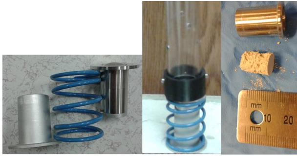
Figure 13. Implemented drive tube components (left) assembled (middle) and sample tube with collected sample (right)
